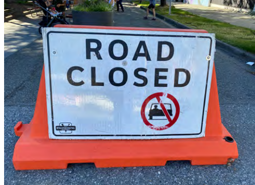
Current examples of plastic jersey barricades and signs used in Vancouver.
