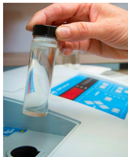
Analysing a water sample using a Spectrophotometer
