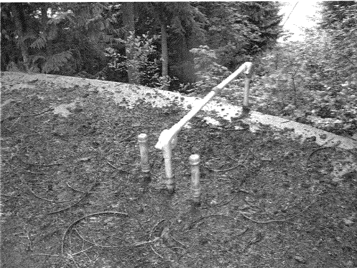
69. Water level indicator housing
