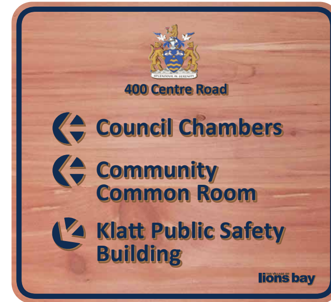
Pantone 295 dark blue text and border on sandblasted cedar 50 cm wide. Corner radius is 5 mm, border width is 1.5 cm. Blind screws from behind thru 4x4 PT wood post. Cedar signs utilise the Coat of Arms rather than the wordmark.
