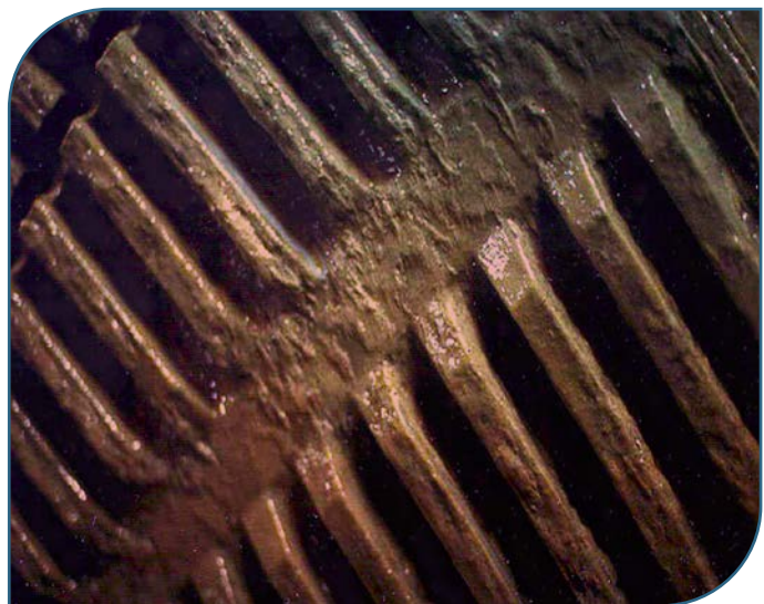
Photo: Initial biofilm growth on RBC media.
