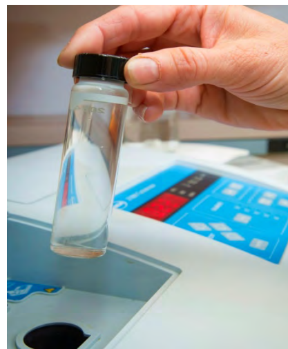
Analysing a water sample using a Spectrophotometer
