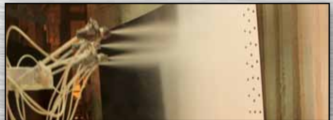
Stage 2: Panels are coated with Vitrium glass coating
