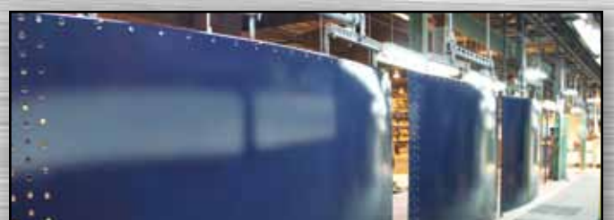
Stage 4: Glass-fused-to-steel sheets are quality tested and prepared for shipment
