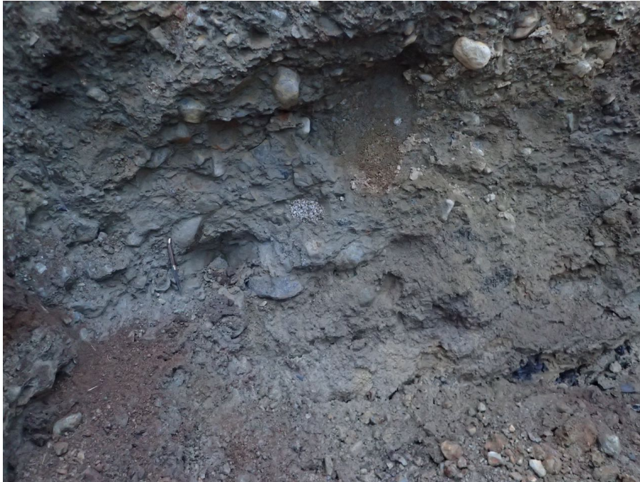
Photo 1. Till in house excavation, Lot 60 Oceanview Road.
