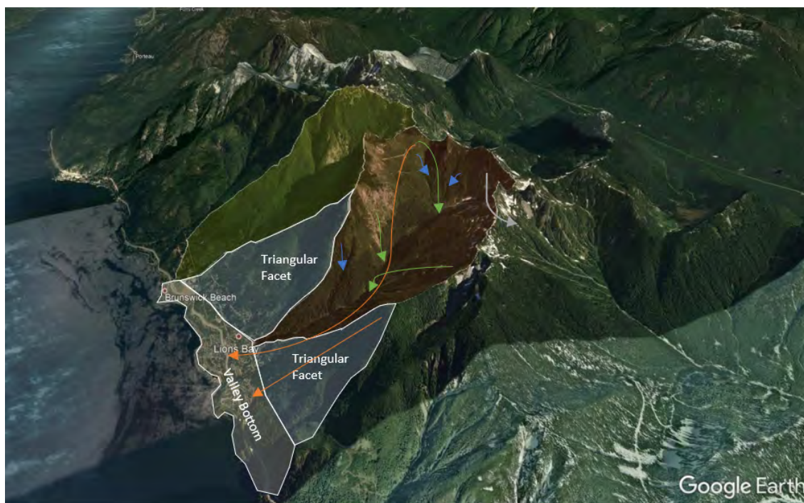
Figure 3.1: Flow pathways in a conceptual model for the flow generation and storage mechanisms
