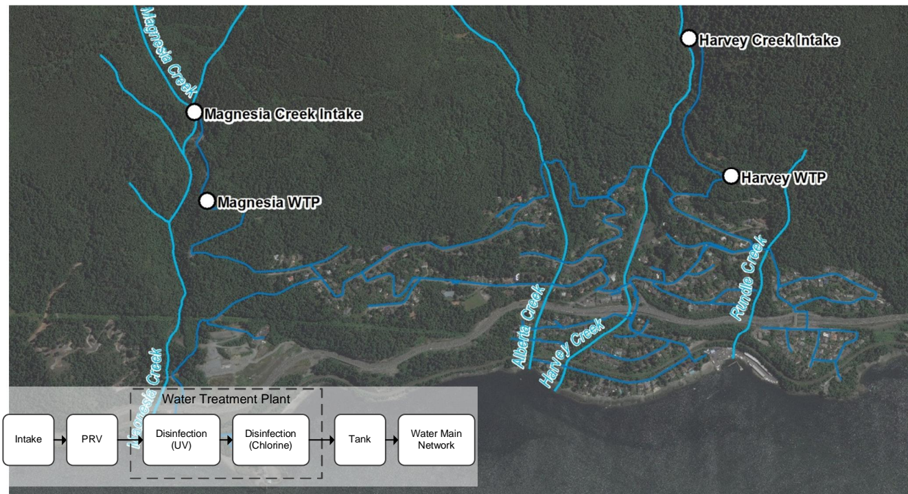
Figure 2-9: Existing Treatment Plants
