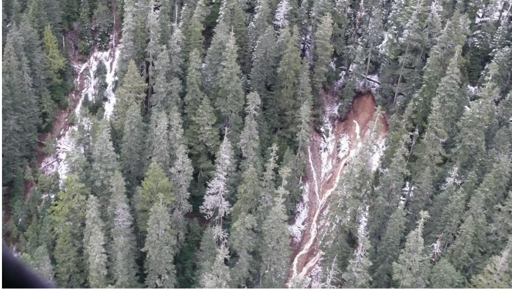
Figure 1: Helicopter inspection after Dec. 2014 major rainfall event showed scouring, landslides and streams piping from the ground
